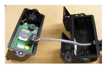
**3.4.** Slide SIM card door backward towards hinges and lift door to open SIM card holder. Remove existing SIM card if applicable. Slide new SIM card into holder observing polarity, close door and slide forward to secure SIM card.
